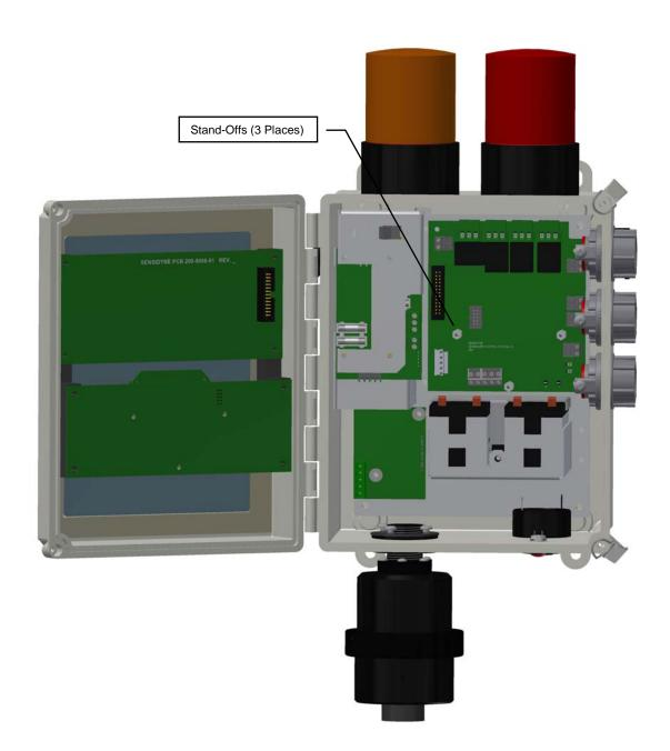
4. Remove HART Connector from Main PCA. Attach wires from **TB9** on Hart PCA (Red Wire from TB9 on Hart Plug to Main PCA (+) Hart Connector Pin) (Black Wire from TB9 on Hart Plug to Main PCA (-) Hart Connector Pin)
